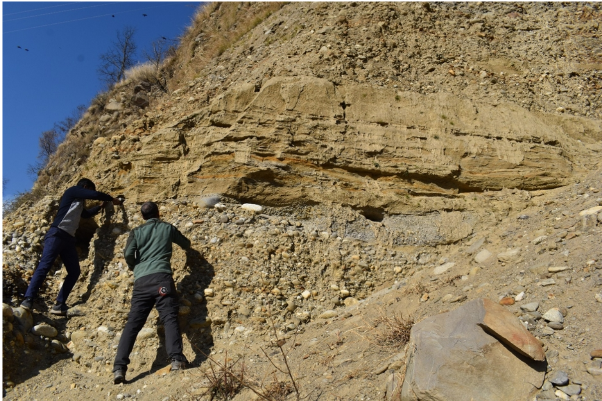
Figure 2 . Researchers are collecting samples from the fill terrace deposits for OSL dating and cosmogenic nuclide analysis.
